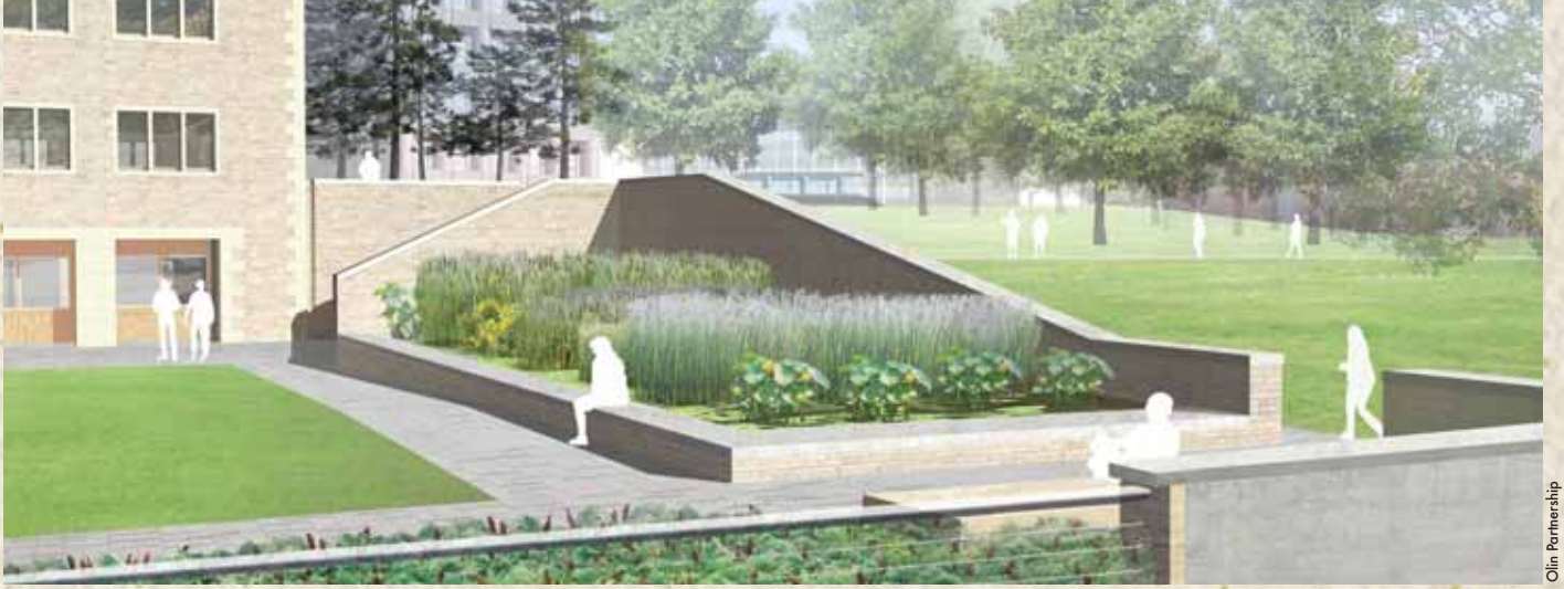
Aquatic plants in the pond, above, will play a crucial role in cleansing stormwater, which will be used for landscape irrigation and toilets.
