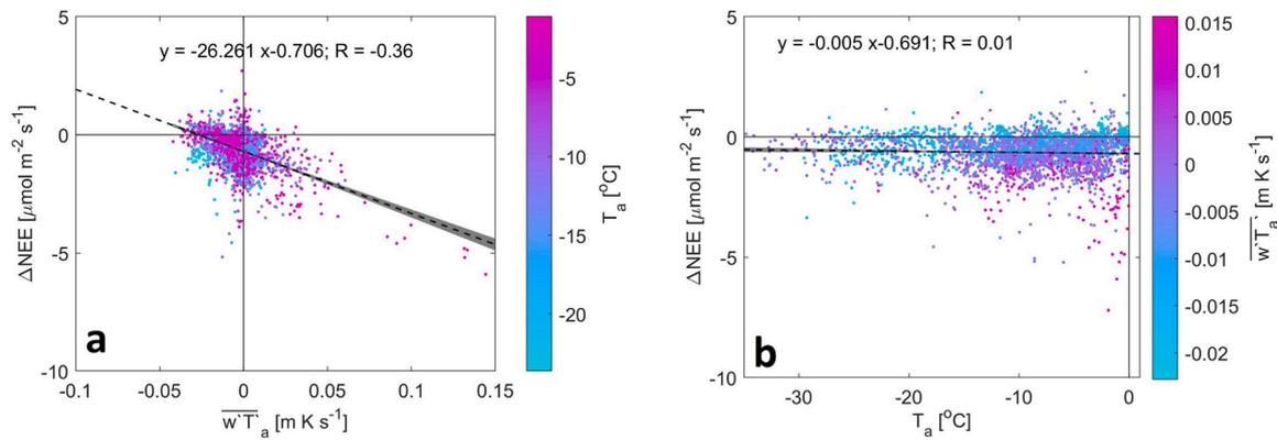
**Fig. 2.** Relationship between absolute flux bias ( $\Delta NEE = F_{OP} - F_{CP}$ ), kinematic heat flux ( $\overline{wT_a}$ ), and ambient temperatures ( $T_a$ ). Data plotted ( $n = 3061$ ) are for the snow-covered season (albedo  $> 0.4$ ) when  $T_a < 0$  °C. Dashed lines and equations represent ordinary least squares regressions with 95% confidence intervals in shaded gray.
