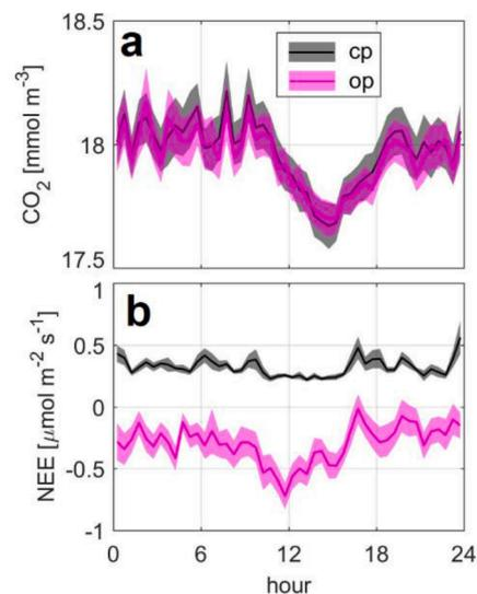
Fig. 7. Panel a shows the median diurnal CO<sub>2</sub> molar densities for the closed-path (black line) and open-path (magenta line) analyzers with standard errors (shaded areas) during December 2018. Panel b shows the corresponding median diurnal NEE values. Despite good agreement in the CO<sub>2</sub> concentration measurements (RMSE = 0.05 mmol m<sup>-3</sup>), the NEE estimates imply fluxes that are opposite in sign, with enhanced biases around noon.
