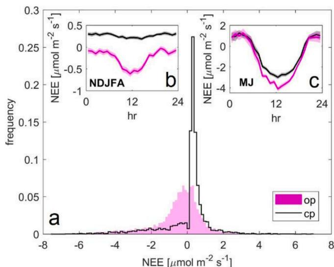
**Fig. 1.** (a) Histograms of  $\text{CO}_2$  fluxes measured with open- (purple) and closed-path (black) analyzers from November 2018 through June 2019 (mean  $T_a = -3.7^{\circ}\text{C}$ ). Panels inset show median hourly fluxes (lines) with standard errors (shaded areas) for (b) November 2018 through April 2019 and (c) May 2019 through June 2019.
