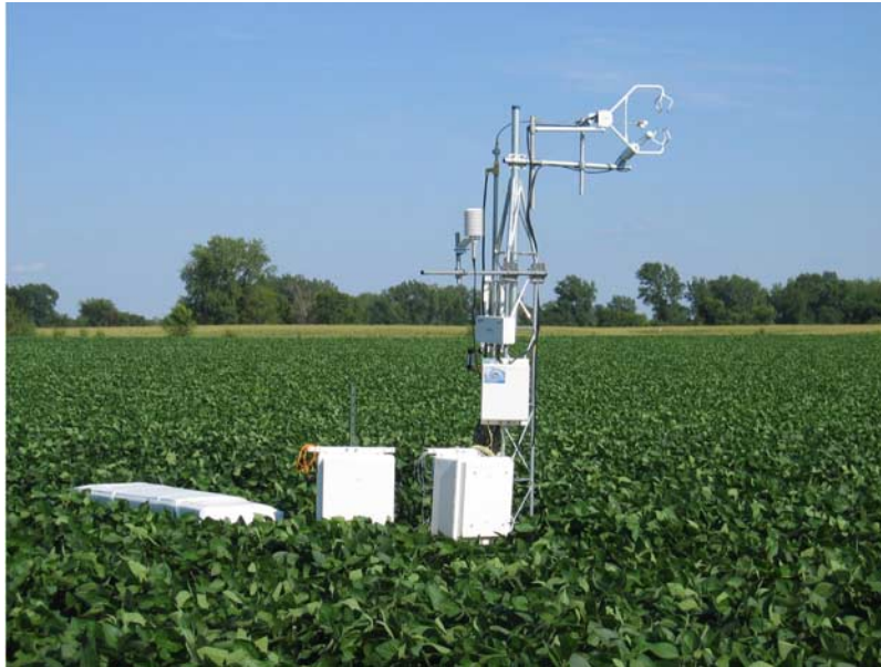
Figure 3. Photograph of the eddy covariance and tunable diode laser (EC-TDL) system deployed at the University of Minnesota, Rosemount Research and Outreach Center, during the 2006 growing season. Isotopic flux measurements were made over a soybean canopy from 18 July to 20 September 2006.
