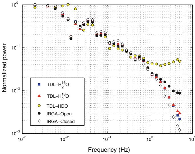
**Fig. 9** Spectral density analysis. Normalised spectrum of TDL and IRGA 10Hz time series over a 3-h period (1200–1500 local time) on DOY 228, 2008 soybean canopy. Spectra were computed at 10-min intervals using Welch’s averages periodogram method using Matlab. The spectra were bin averaged using 10 logarithmically spaced intervals per decade. Wind direction was 150° from north and wind speeds were approximately 1.5 m s<sup>-1</sup>. *F* ranged between 8 and 9 mmol m<sup>-2</sup> s<sup>-1</sup>
