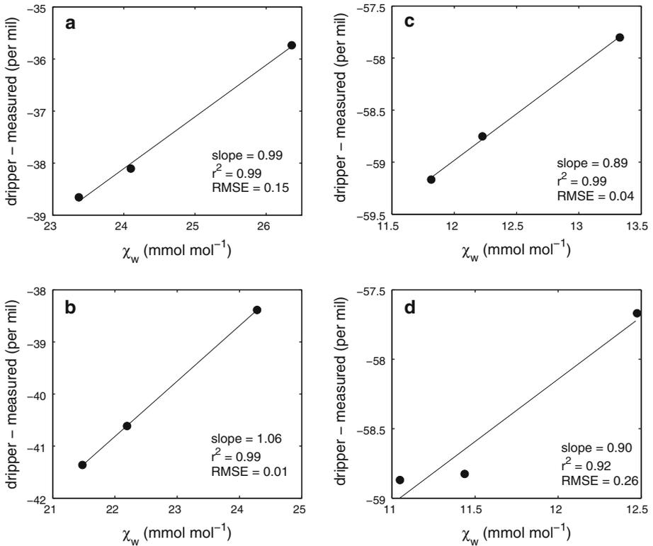
**Fig. 7** Examples of the typical range of calibration correction factors and their dependence on the water vapour mixing ratio. The values shown are median hourly values for typical days during the 2009 corn field experiment. These values are corrected for a zero offset. A gain correction was not applied
