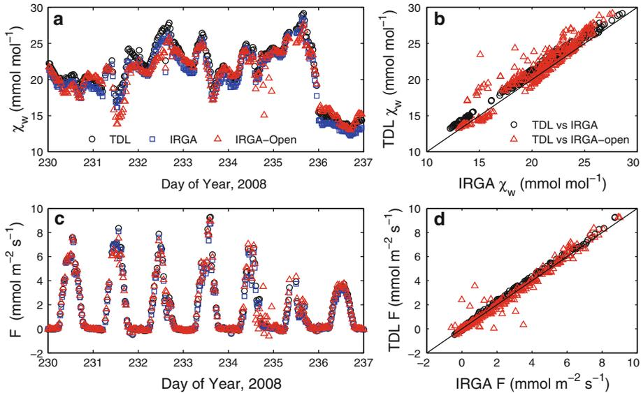
**Fig. 8** Time series of water vapour mixing ratio measured with the TDL, IRGA, and open-path IRGA (a) and their 1:1 comparison (b); time series of the water vapour flux measured over the soybean canopy using eddy covariance based on three methods including the TDL, IRGA, and open-path IRGA (c) and their 1:1 comparison (d)
