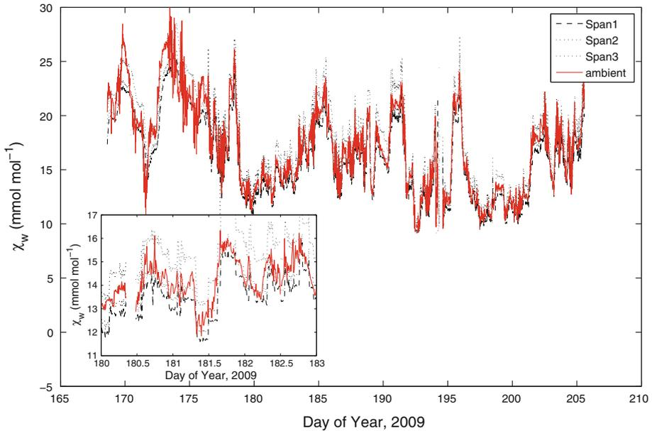
**Fig. 2** Time series of the dynamic water vapour mixing ratio calibration for the 2009 corn growing season. Three span values were used to bracket the ambient water vapour mixing ratio by adjusting the pressure set point of the calibration dripper device. The *inset* shows a magnified view of the time series from DOY 180 to DOY 183 where the ambient mixing ratio was bracketed to within  $1 \text{ mmol mol}^{-1}$
