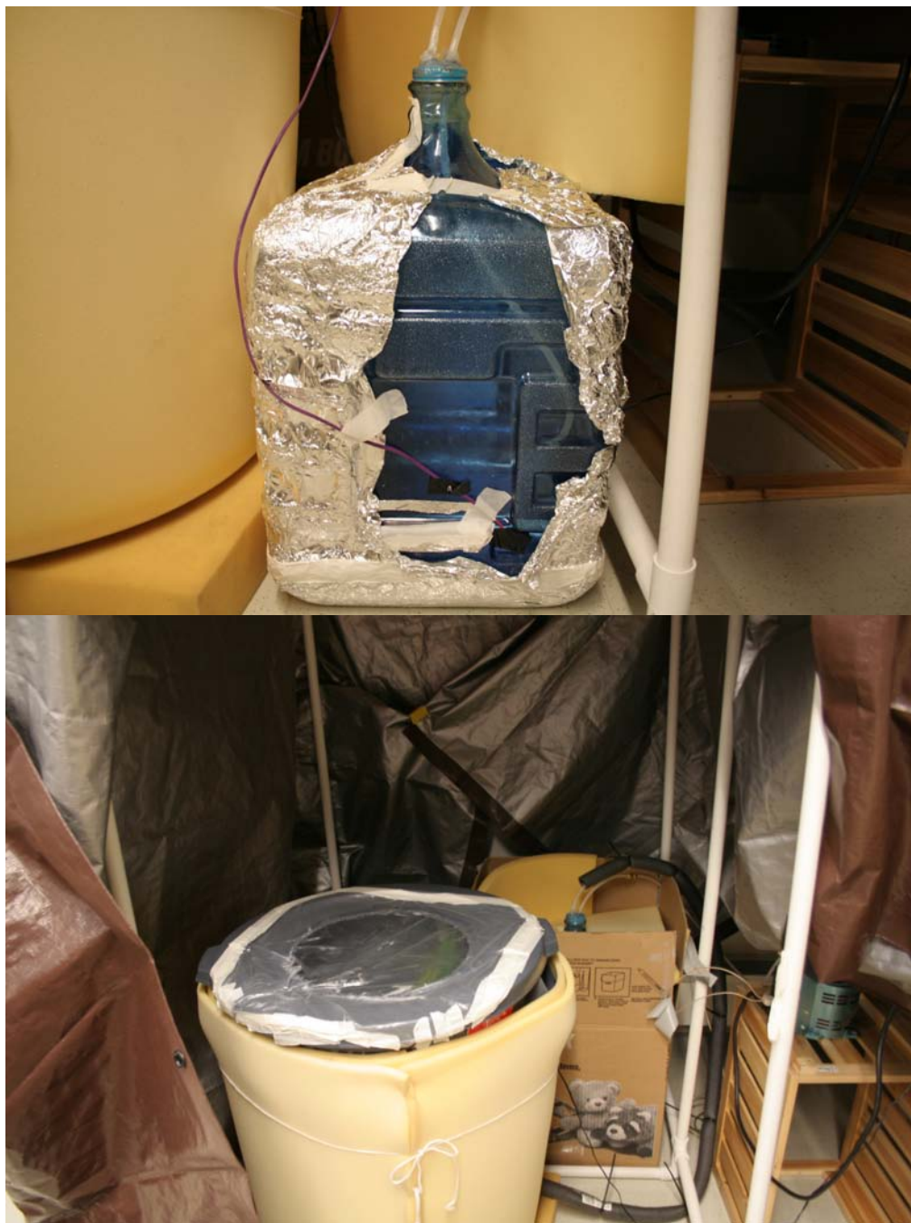
Photo A3.5. Laboratory set-up for the fumigation experiment in Chapter 3. The bubbler (upper) and the plant chamber (bottom).
