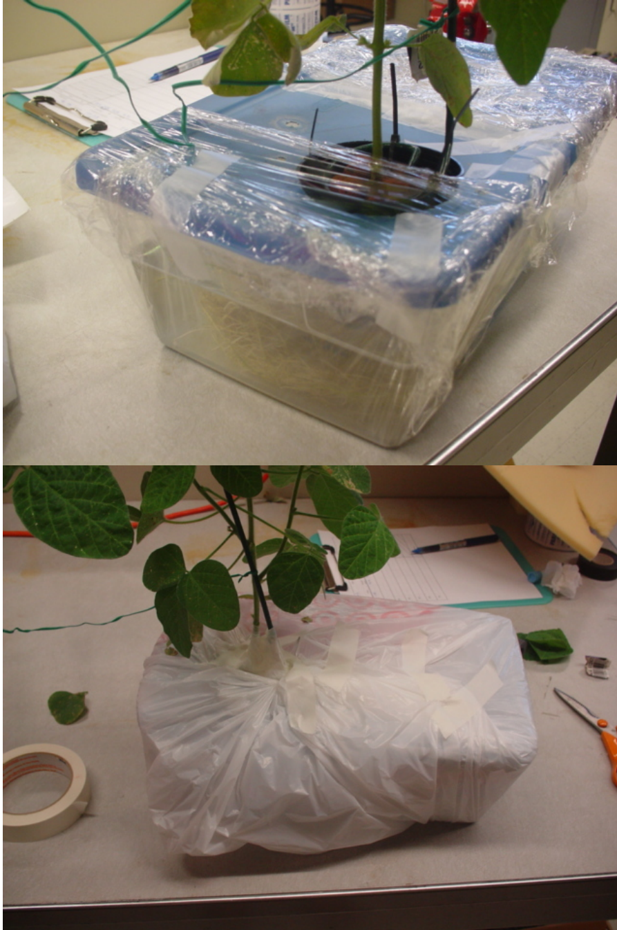
Photo A3.4. Plant source water was carefully sealed prior to the fumigation experiment (Chapter 3) in order to prevent from contaminating fumigation vapor.
