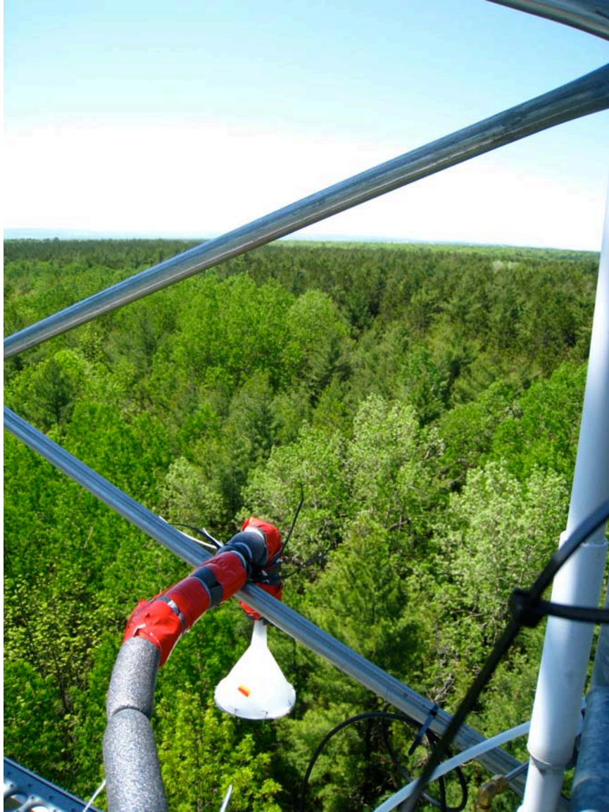
Photo A3.6. Field set-up at the Borden site, Ontario, Canada (Chapter 4). An intake of ambient air installed at a flux tower.
