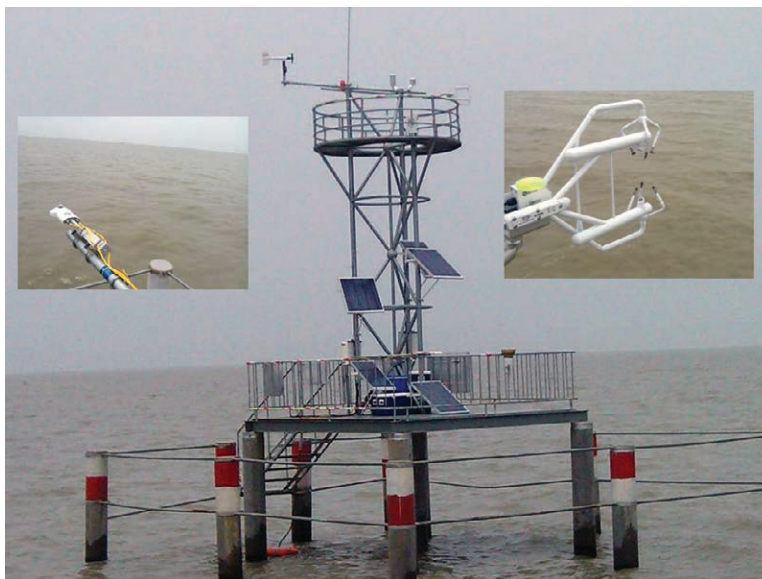
FIG. 2. The PTS instrument platform in zone 4 (Fig. 1). Insets are photos of the (left) four-way radiometer and (right) eddy covariance sensors.
