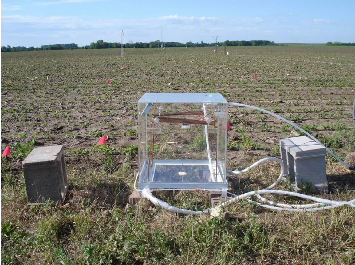
Figure A1.3. Chamber blank test set-up. A blank test was conducted for the medium chamber at the beginning of the growing season, by measuring the \text{CH}_4 and \text{N}_2\text{O} concentration from the inlet and outlet of the chamber without enclosing plants in it. The hole at the center of the bottom plates was designed to allow the plant stem to pass through, but it was sealed during the blank test. Three small towers were set up in the field for different measurements. The middle tower was equipped with a closed-path \text{CO}_2 eddy covariance system. Air was drawn at two levels of the towers at the edge of the field for continuous \text{N}_2\text{O} concentration analysis. As a result, \text{N}_2\text{O} flux from the soil-plant ecosystem was determined (Chapter 3). \text{N}_2\text{O} concentration was measured by TDL.
