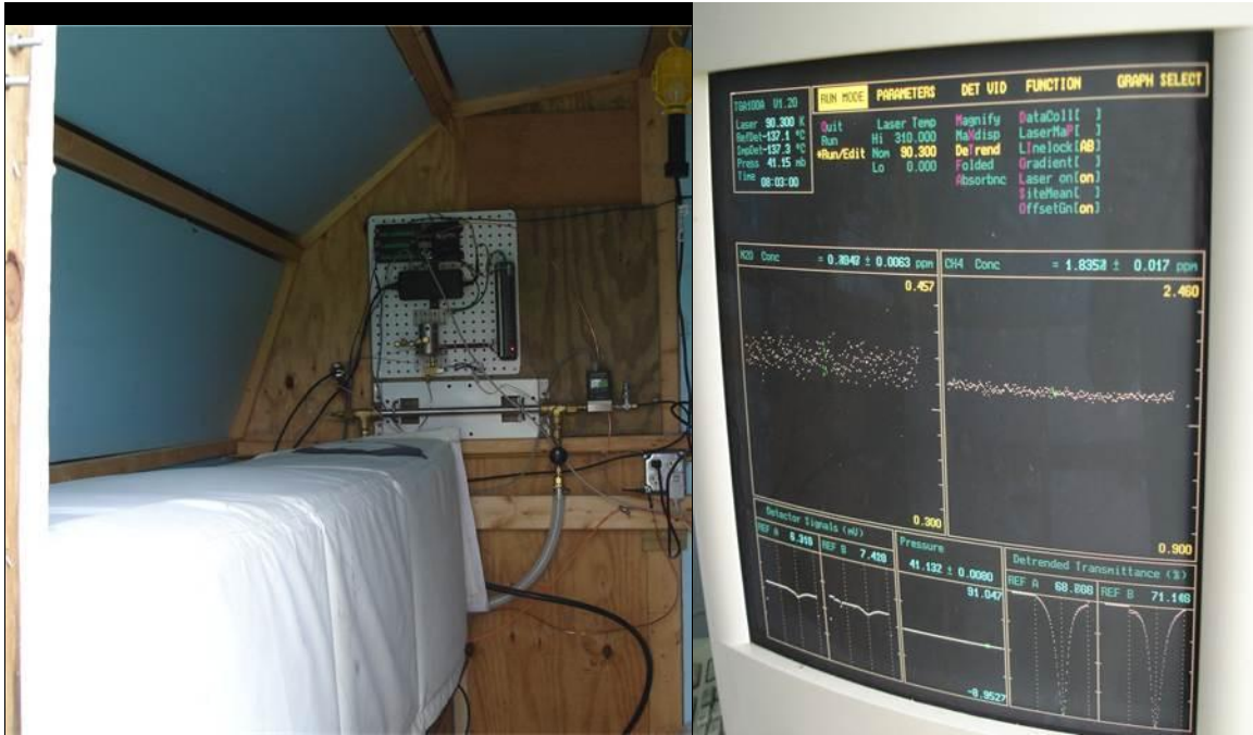
Figure A1.7. The setup of TDL sampling system and a screenshot of TDL measurement.
