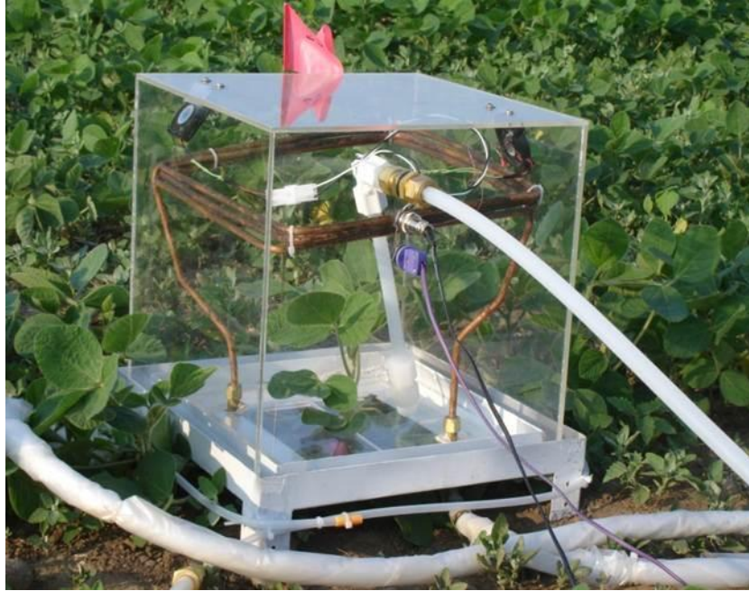
Figure A1.4. Soybean plant flux measured by the small chamber. Soybean plant flux was measured in the small chamber by enclosing the aboveground section of the plant inside the chamber. Ambient air was allowed to flow into the chamber from the bottom, and \text{CO}_2 , \text{H}_2\text{O} , \text{CH}_4 and \text{N}_2\text{O} concentrations were measured.
