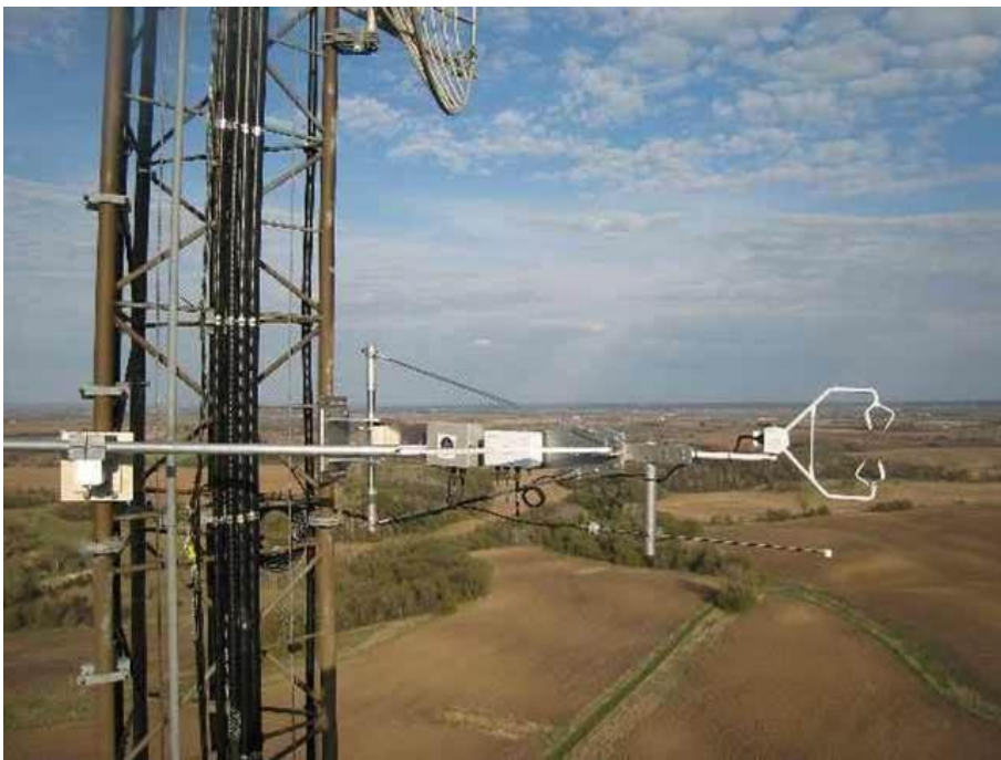
Figure A1.9. Tall tower observatory. The upper panel is the setup of LI-COR and TDL for measuring trace gas concentration from the air samples from 3 m and 200 m during the intensive campaign in 2009. The lower panel is a snapshot of the view from the 100 m level at the tall tower. The equipment attached to the tower is a 3-D sonic anemometer-thermometer (model CSAT3, Campbell Scientific) for eddy covariance measurement.
