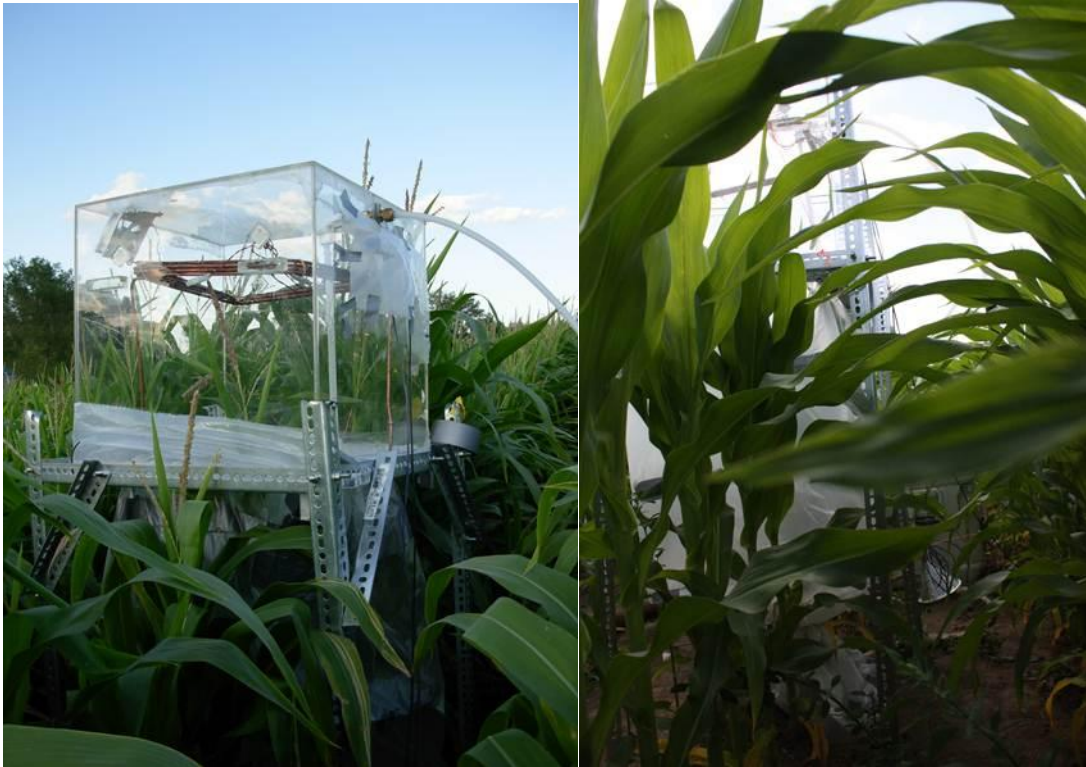
Figure A1.5. Corn plant flux measured by the large chamber. Corn plant flux in the late growing season was measured by the large chamber, which consisted of the medium chamber with its bottom cover plates removed and a skirt made of transparent polyethylene sheets. The plexiglass part rested on a metal frame of adjustable height, ranging between 1 m and 1.7 m. The polyethylene skirt was attached to its side by a strong bonding tape. The contact of the skirt and the medium chamber cover was sealed by water kept in the base frame. The bottom of the skirt was loosely tied to the base of the plant allowing air to enter from the base of the plant.
